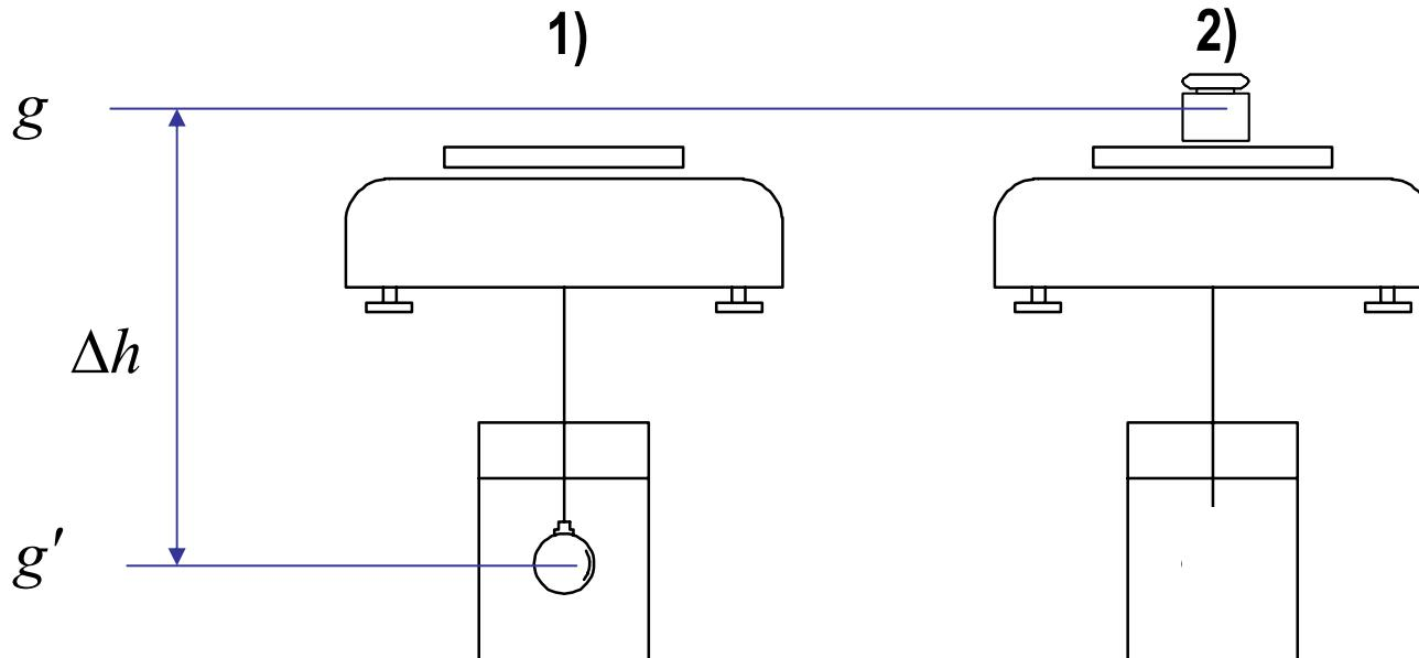
$$1) \quad I_{ds} k\theta = g' \cdot \left[ m_{ds} - \rho_L V_{ds} \cdot [1 + \alpha_{ds}(t_{liq} - t_{ref})] \cdot [1 - \beta_{ds}(p_{liq} - p_{ref})] + \left( \frac{\pi \gamma_{liq} d}{g'} \right) \right]$$
